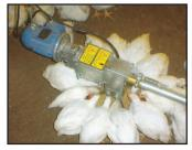
The control unit's low volume ensures frequent operating of the feeding system thus stimulating the feed consumption.
